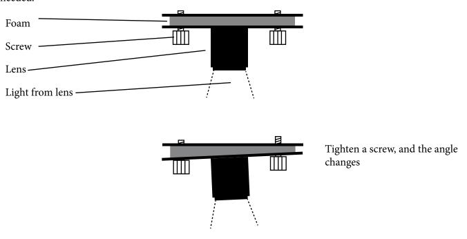
Take a look at a standard lens board - simple, flat piece of aluminum in most cases, with an opening for the lens, surrounded by a recessed edge. The recess is for the lens retaining ring. It's not 100% necessary, but usually there.
