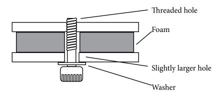
The length of the screw is important, in that it shouldn't protrude too far up into the lens stage to interfere with any enlarger parts, but should give you at least a 1/8" or so adjustment range.
