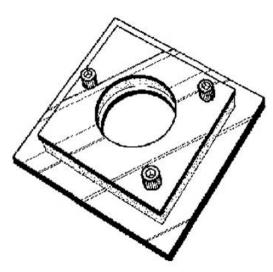
The board is essentially two lens boards, with black foam - about the thickness of a mouse pad or yoga mat - sandwiched between them. Three screws allow you to tighten or loosen the setup, to cover any possible angle needed.
